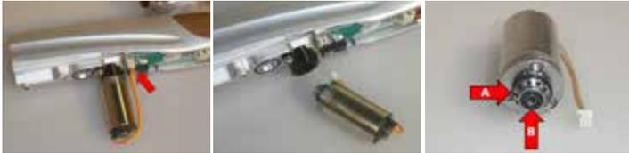
4. Inspect each O-ring at the bottom of Solenoid threads (labeled A) and the top of Solenoid (labeled B) for damage, replace as necessary (see Figure 6c).
