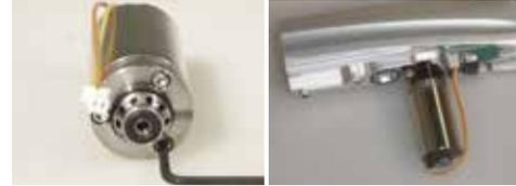
**WARNING: Solenoid may be in open position after service. Before gassing up marker, turn marker on, turn eyes off and pull trigger several times to close solenoid**
